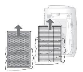
**3** Place the Filter within the main unit. Do not install the filter backwards or the product will not operate properly.
