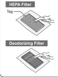
Gently remove dust from HEPA Filter and Deodorizing Filter with a vacuum cleaner attachment or similar tool.
